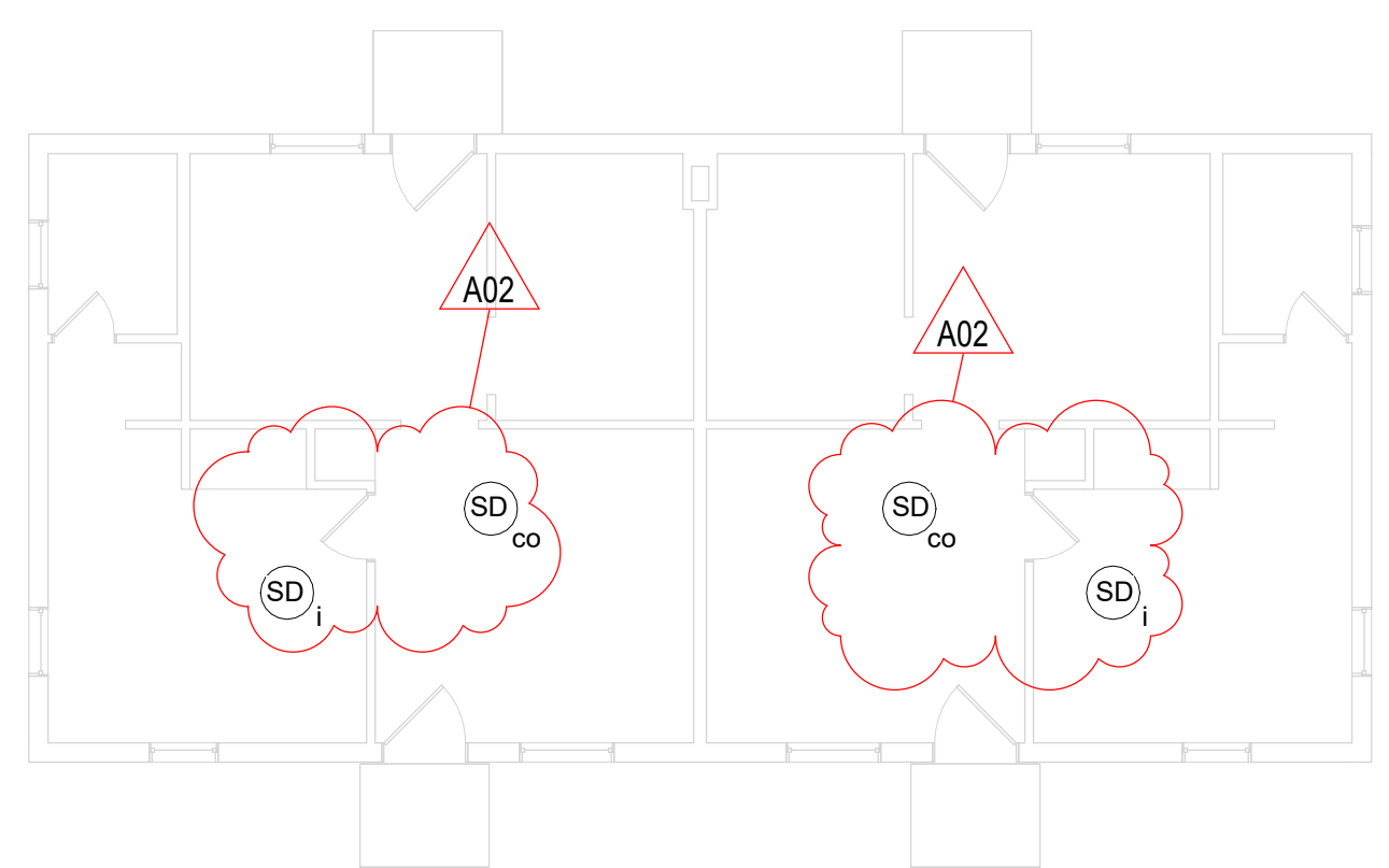
1 1ST FLR A1 BLDG SMOKE ALARM PLAN 1/8" = 1'-0"
